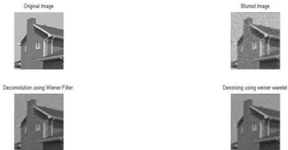
Fig 4. Image deblurring on gray image House (256x256) with Wavelet and Wiener
